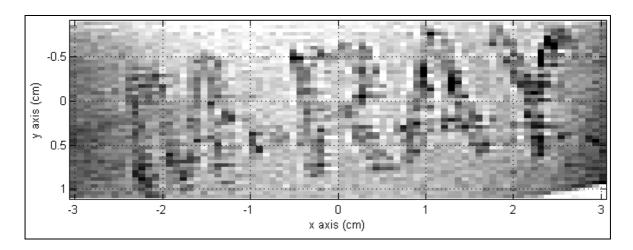
The slide was made by laser etching "M-RAY" the glass slide, and then immobilising cDNA into the etch surface before hybridising with cDNA (as described in the communication) and imaging in water. MRI details: RARE sequence, RARE factor = number of lines = 128,  $T_E = 30~ms, \ T_E^{eff} = 1726~ms, \ 16$  averages, spatial resolution = 781 x 391  $\mu m^2$ , slice thickness = 1 mm, imaging time = 62 s.
