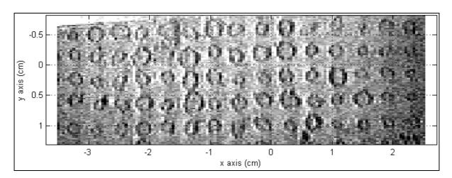
The slide was made by laser etching a 5 x 15 array and spotting with cDNA (all the same). cDNA was then spotted onto the spots directly and allowed to dry. This was subsequently washed before imaging in water. MRI details: RARE sequence, RARE factor = number of lines = 64,  $T_E$  = 30 ms,  $T_E^{eff}$  = 975 ms, 8 averages, spatial resolution = 1172 x 547  $\mu m^2$ , slice thickness = 0.5 mm, imaging time = 15.5 s.
